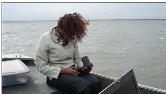
Figure 6. Martha Ragwa of JSU is taking turbidity measurement using a HACH colorimeter.
